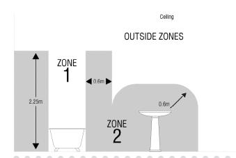
This product is suitable for use in Zone 1, Zone 2 and outside Zones of a bathroom. See diagram. If this unit is being fitted in a room containing a bath or shower, a 30mA RCD must be used, in accordance with IEE regulations.
